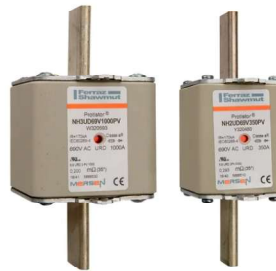
NH Square Body High-Speed Fuse Protistor AC Protection 690VAC (IEC) / 700VAC (UL) Protistor® size NH 000, 00, 0, 1, 2, 3 aR,
